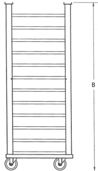
Glides are 1" x 2" x .080" thick extruded aluminum welded front and back to the frame
